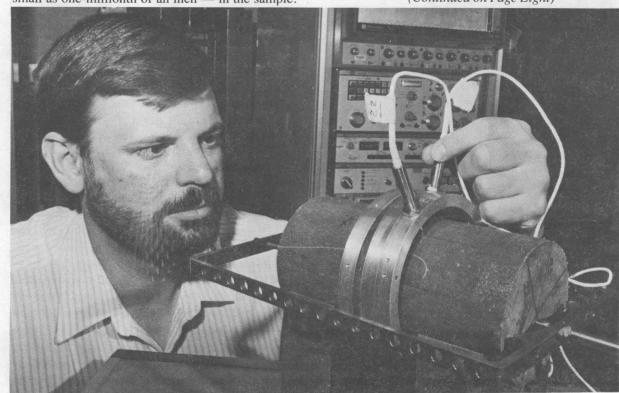
LARRY TEUFEL (6232) adjusts a linear variable displacement transducer (LVDT) on the special ASR tool used to detect strain displacement movements in a core sample.
